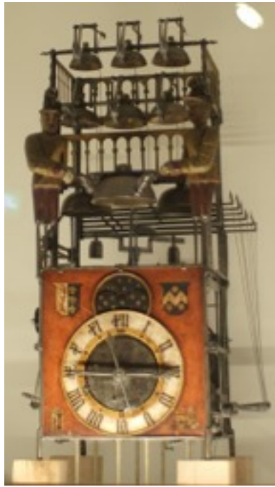
Jacks strike the bell on this Medieval clock from the Netherlands, 1450-1550. The clock is now in the collection of the Museum Speelklok, Utrecht, Netherlands.
